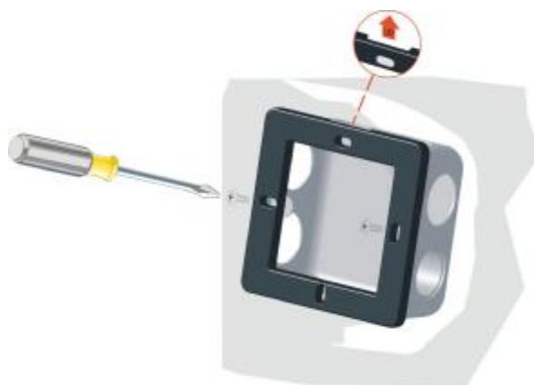
Fig.2: Mount the plate
