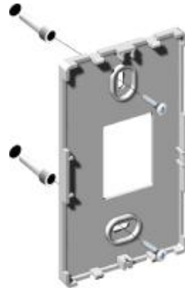
Fig. 4. Installing back plate
