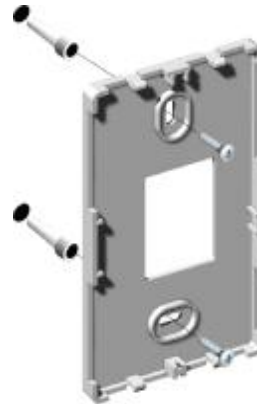
Fig. 4. Installing back plate
